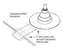
Apply ClassicBond uncured T-Joint Patches where pipe seal intersects a field splice.
